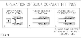
**Stream Height Adjustment:** Stream height is factory set at 35 PSI. If supply pressure varies greatly from this, adjust screw on item 20, by using a small screw driver through the small hole in the push button (Item 10). Clockwise adjustment will raise stream and counter-clockwise adjustment will lower stream. For best adjustment, stream should hit basin approx. 6-1/2" from bubbler.
